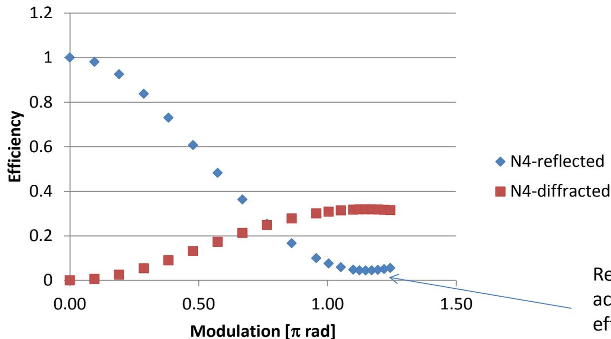
Real grating can never achieve 100% diffraction efficiency => Poor contrast
