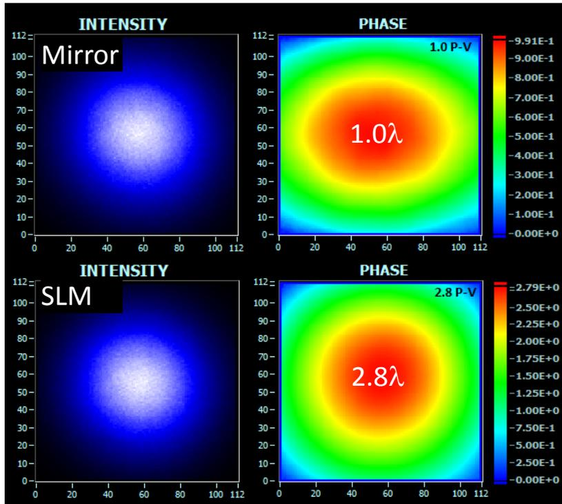
SLM adds constant wavefront aberration of  $1.8\lambda$ , but most of it is defocus.
