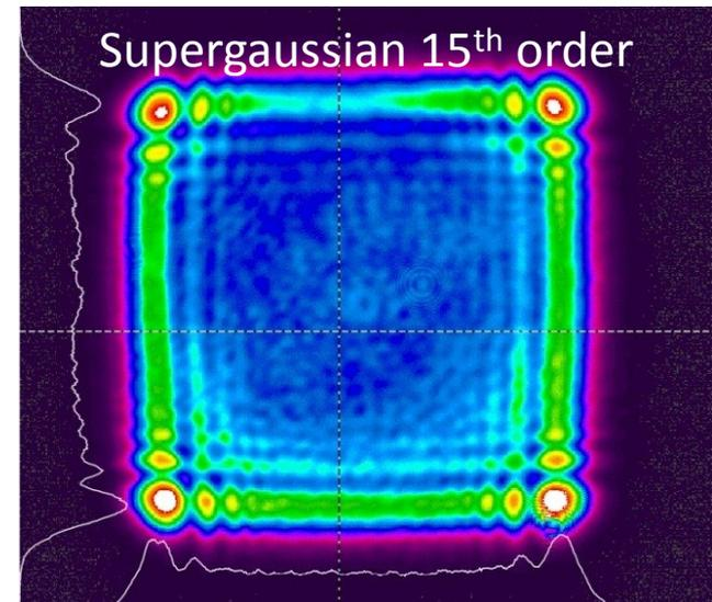
Diffraction effect modulates beam in just  $1f$  distance from image plane (beam size  $10 \times 10$  mm,  $f = 100$  mm).
