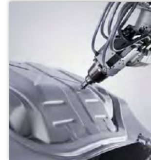
Right: Thin-disk, laser-pumped high-brightness fibre laser developed at the IFSW for material processing applications. © IFSW, University of Stuttgart
