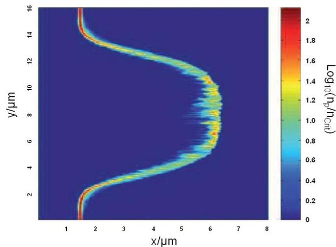
**Figure 2 – Computer simulation of an ultrathin foil irradiated by a circularly polarized laser pulse [9]. The whole foil is accelerated in the x direction (the laser propagation axis) by the incident laser radiation pressure. The use of circular polarization inhibits hot electron generation, effectively switching the regime from TNSA to RPA.**
