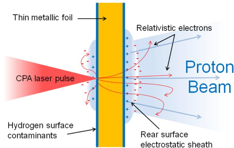
**Figure 1 – Schematic of the proton acceleration from thin foils via target normal sheath acceleration (TNSA). Hydrogen surface contaminants on the foil surface are most readily accelerated in the sheath field set up at the plasma vacuum boundaries. As the boundary is sharpest at the rear unirradiated side, protons from this region achieve the highest energies and exhibit unrivaled laminarity.**
