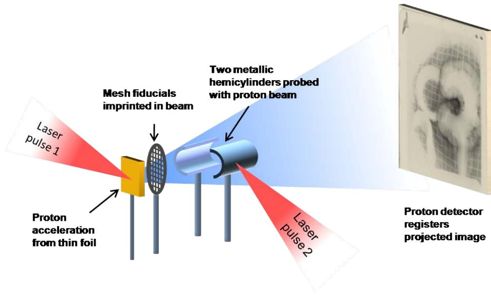
Figure 3 – Proton imaging of the picosecond dynamics of laser plasma interaction: the hemicylinder on the right is irradiated with an intense laser beam, heating electrons and generating strong electrostatic fields at the target-vacuum interface, which deflect the probe particles. This causes the halo effect around the target in the detector image. These fields decay over a few tens of picoseconds. Figure adapted from [13].
