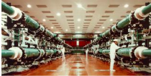
Gekko XII (Osaka, Japan, 1983) 25kJ, 0.53 \mu\text{m} , 12 beams 600 times of solid density
