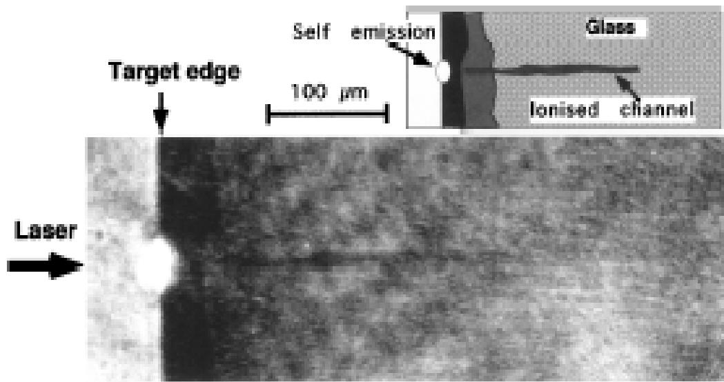
FIG. 2. Shadowgram taken during the interaction of a 20 TW, 1 ps pulse with a solid glass target coated with 1  $\mu\text{m}$  of Al.
