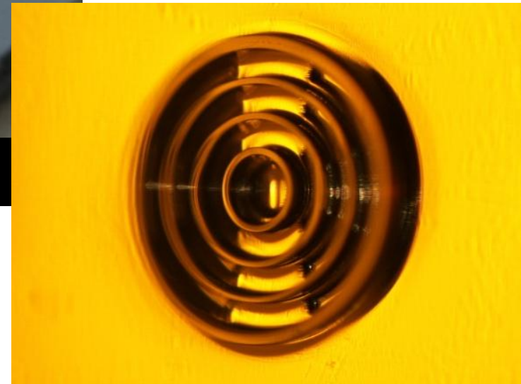
Complex nozzle fluidics Core + 3 shells
