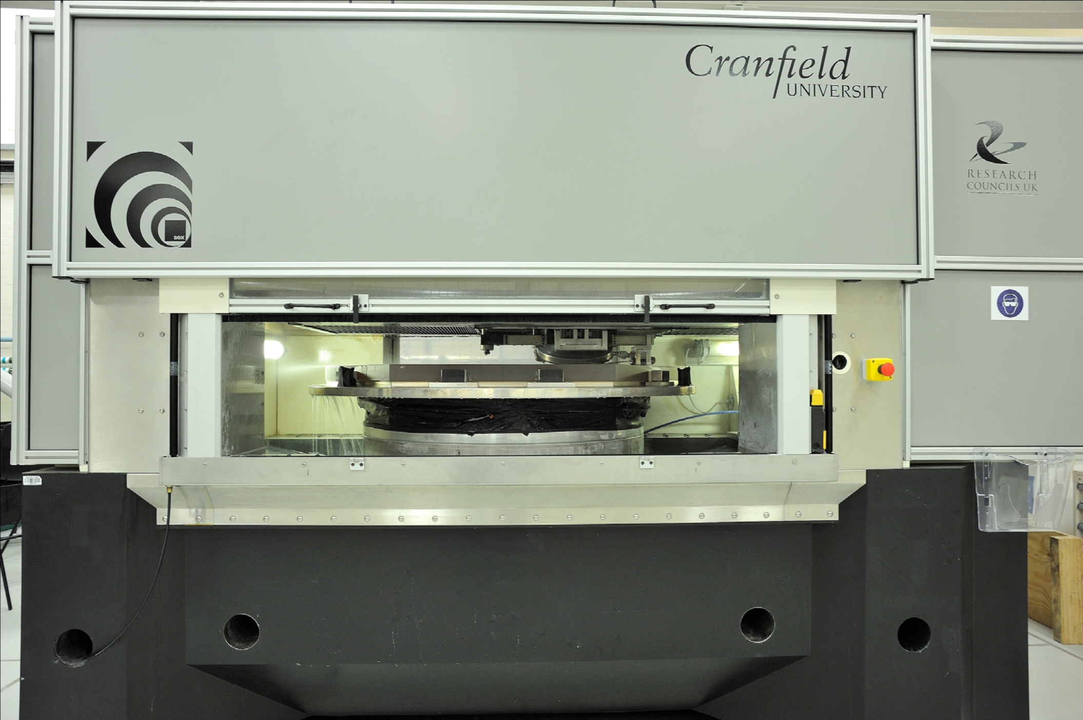
Box machine grinding 1 st ESO segment
