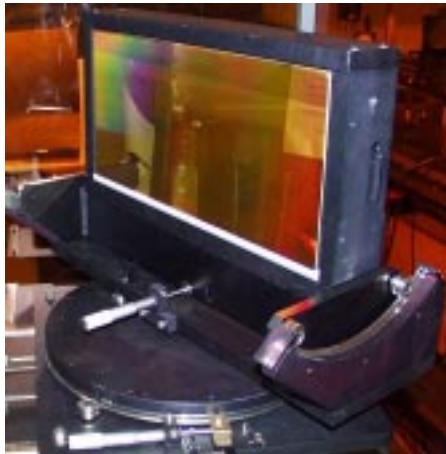
Figure 1. 420 mm x 210 mm Diffraction Grating
