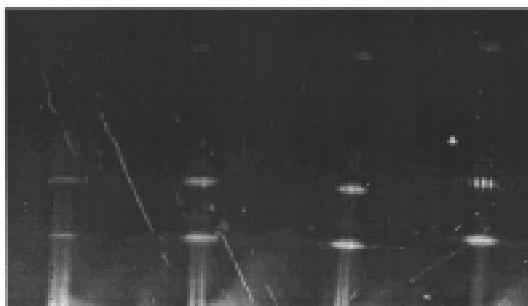
Figure 3. Experimental fringe distributions for 23.2\ \text{nm} and 23.6\ \text{nm} radiation and the diagnostic of figure 2.
