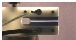
Figure 1: York atmospheric-pressure plasma jet.
