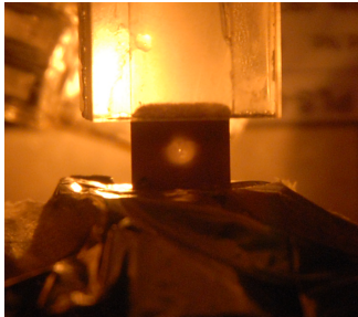
Cryogenic deuterium target irradiated by two high energy laser pulses. [J. Menzel]
