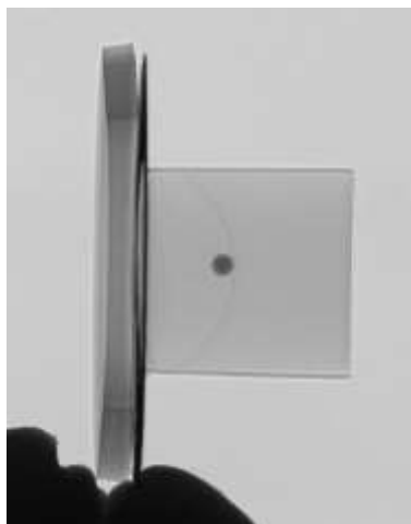
Figure 4. Side on radiograph of ruby embedded in TMPTA foam showing a slight interfacial membrane.
