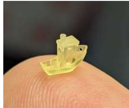
Figure 1. Example of a test print. 3DBenchy is a widely-used test object designed to evaluate accuracy of 3D printers.
