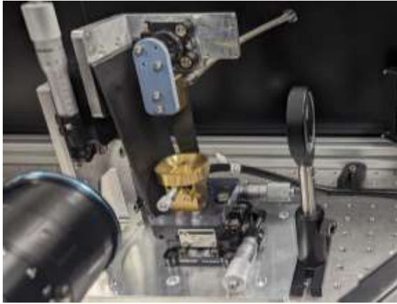
Figure 2. The liquid target nozzle and catcher system
