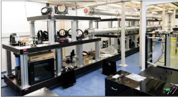
Figure 3: 3-tier table installed in LA4. A large-aperture (90 mm) LBO OPA stage on the bottom level will be pumped by a frequency-converted Vulcan long pulse beam, delivered from the top level.
