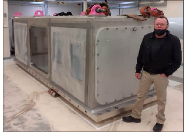
Figure 4: CLF’s Simon Spurdle beside the new ‘compact’ VOPPEL compressor chamber based on the Gemini double-pass design, aimed at compressing the large bandwidth pulse to 20-25 fs with \sim 67\% efficiency.
