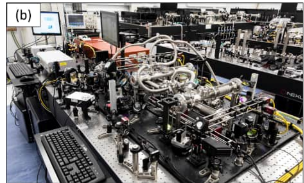
Figure 2: Picosecond front end of the VOPPEL beamline. (a) Stages 1 & 2, (b) Stages 3 & 4.
