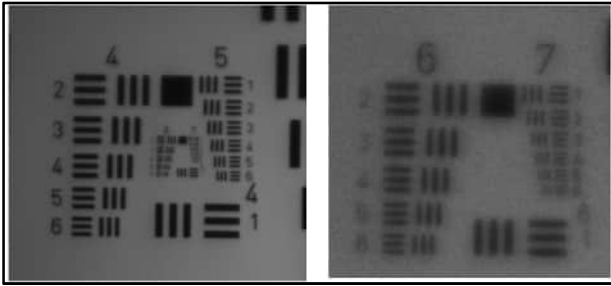
Figure 9. Images of USAF 1951 resolution target taken with the developed high magnification system. LEFT: elements 4 to 7; RIGHT: elements 6 and 7 (digital zoom).
